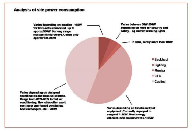
Figure 5 -Analysis of site power consumption<sup>12</sup>
